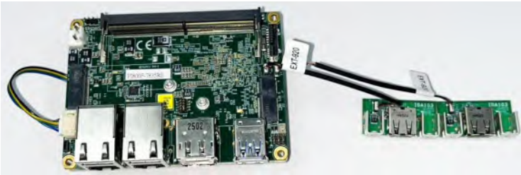
The picture shows EXT-920 cables connected to the J7/J8 headers and to the IDA103 USB 2.0 modules
