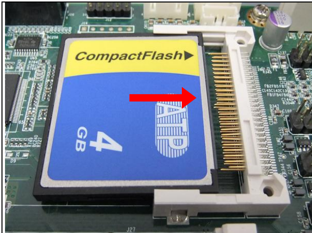
Fig. 7-1 Insert CompactFlash Card into the CF interface
