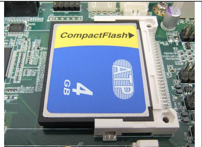
Fig. 7-2 Completion of CompactFlash Card connection
