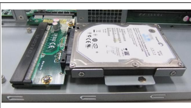
Fig. 9-4 Completion of HDD connection
