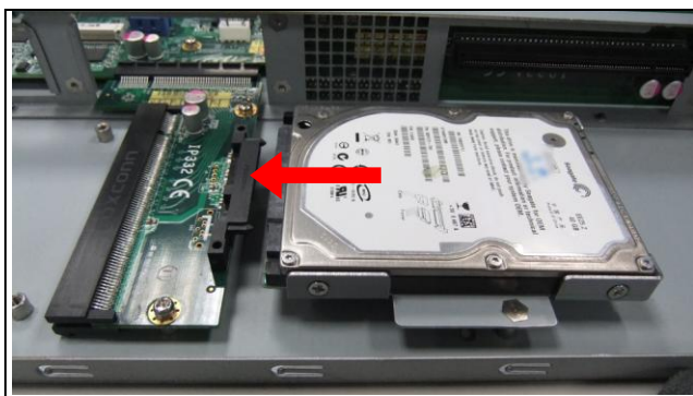
Fig. 9-3 Push HDD into connector
