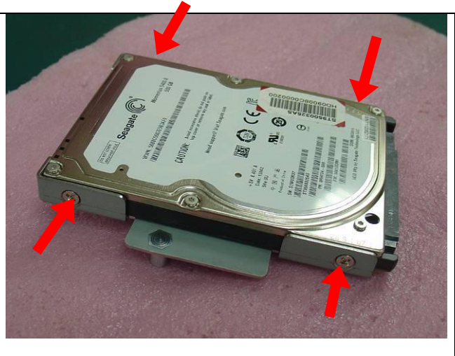
Fig. 9-2 Fasten the four screws to lock HDD and bracket together.
