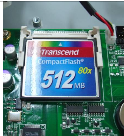
Fig. 7-2 Completion of CompactFlash Card connection
