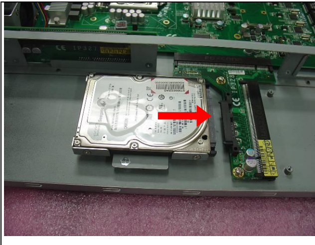
Fig. 9-3 Push HDD into connector
