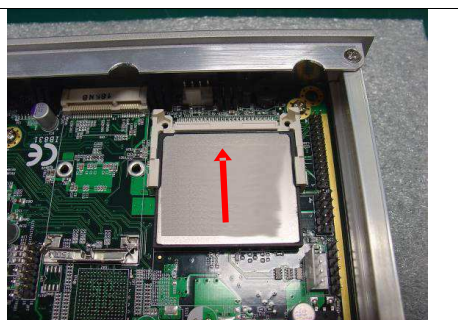
Fig. 6-2 Push Compact Flash Card into the CF interface
