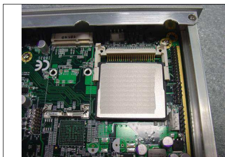
Fig. 6-1 Insert Compact Flash Card
