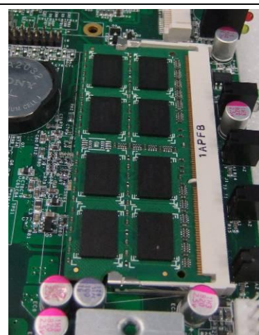
Fig. 7-2 Press down the memory module into socket
