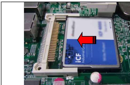
Fig. 6-1 Insert Compact Flash Card
