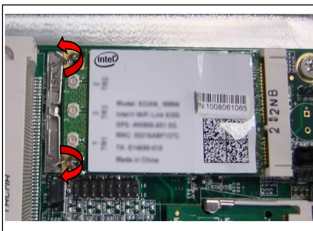
Fig. 9-3 Release two clips to remove module
