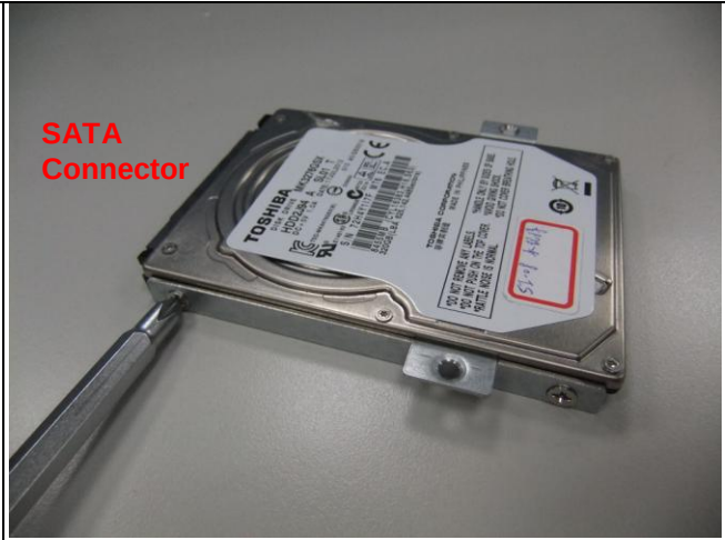
Fig. 8-2 Fasten brackets on SSD with four screws
