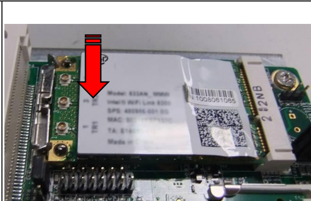
Fig. 9-2 Push down the module into socket
