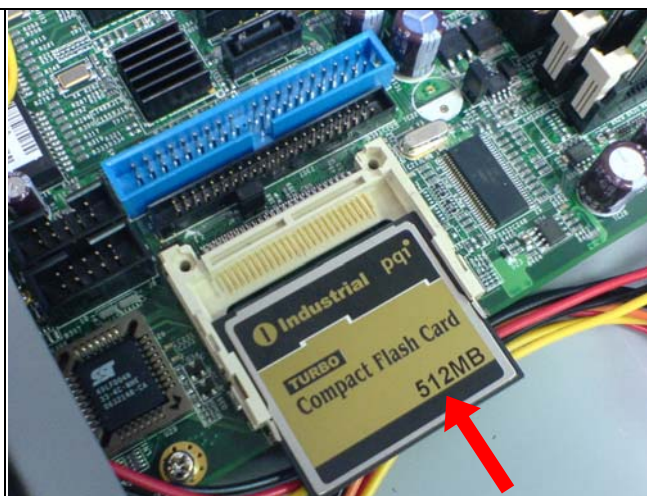
Fig. 7-2 Insert Compact Flash Card into the CF interface
