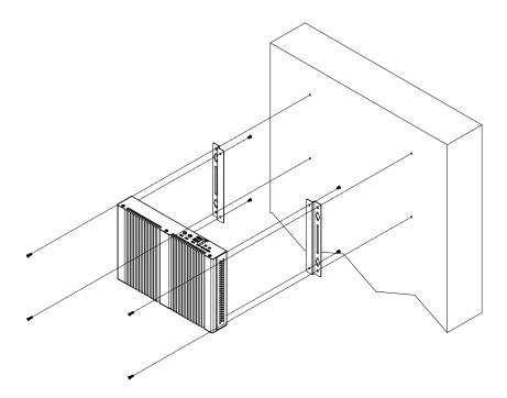
Using attached mounting rail, you can install ASB200 on wood, drywall surface over studs, or a solid concrete or metal plane. Ensure the installer uses at least four M4 length 8mm screws to secure the system on wall. Six M4 length 8mm screws are recommended to secure the system on wall.
