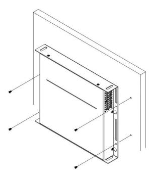
You can install SI-28 on wood, drywall surface over studs, or a solid concrete or metal plane directly. Ensure the installer uses at least four M3 length 8mm screws to secure the system on wall. Six M3 length 8mm screws are recommended to secure the system on wall.
