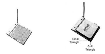
Note: Ensure that the CPU heat sink and the CPU top surface are in total contact to avoid CPU overheating problem that would cause your system to hang or be unstable.
