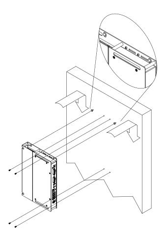
You can install SI-24 on wood, drywall surface over studs, or a solid concrete or metal plane directly. Ensure the installer uses at least four M3 length 8mm screws to secure the system on wall. Six M3 length 8mm screws are recommended to secure the system on wall.
