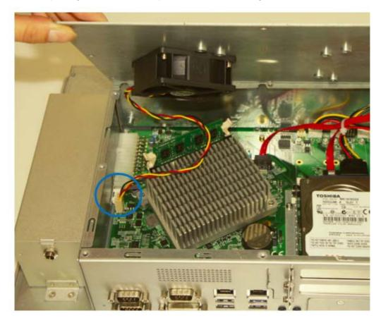
2. After opening the back cover, please note the mating fan cable as shown.
