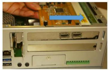
4. Put on the PCI cover bracket and lock the screw.
